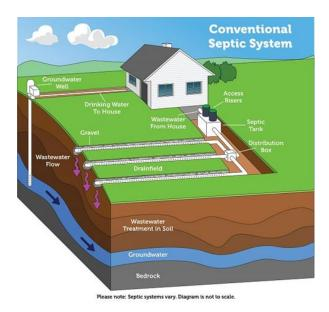
In a conventional OSTDS, a septic tank does not reduce nitrogen from the raw sewage. Approximately 30-40 percent of the nitrogen levels are reduced in the drainfield of a system that is installed 24 inches
